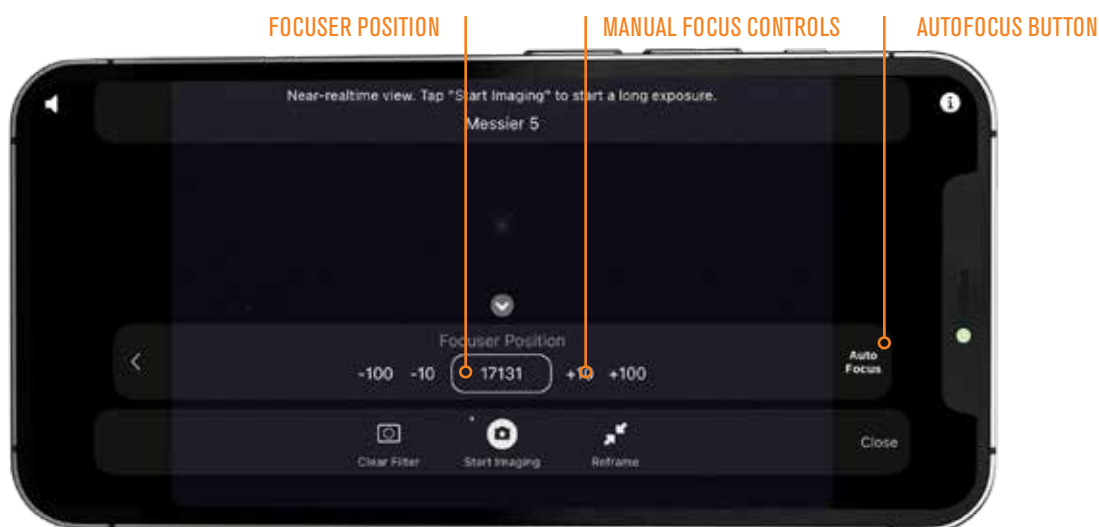
Fig. 12: Use the focus icon to access autofocus and manual focus controls. The Focuser Position can also provide useful information.
