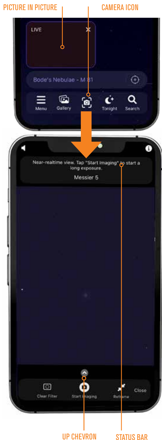
FIG 6: The Camera View is where you observe objects being imaged. It's also where you can access the manual camera controls by tapping the up chevron.
