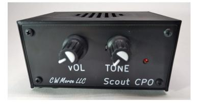
Practice morse code with a straight key and this simple code practice oscillator. Like the old Boy Scout signal training sets of the 1930's, this CPO produces both sound as well as light from the front and back. The CPO has adjustable volume and tone controls from 300-1000Hz along with a headphone jack for private listening. It can also drive a positive keying transmitter up to 30V/500mA with the key jack. SMD parts are pre-soldered, just complete the through hole components.
