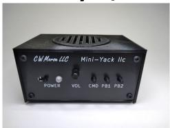
Mini-Yack2c is a basic Iambic keyer based on the open source DK3LJ Yack engine and enhanced with additional features:
