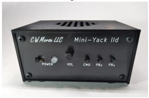
Mini-Yack 2 is a basic Iambic keyer based on the open source DK3LJ Yack engine and enhanced with additional features:
