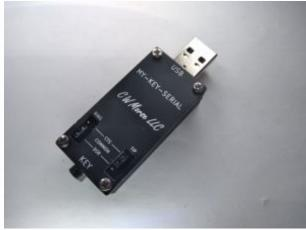
**NEVER plug anything other than a key into the MY-KEY-MOUSE or MY-KEY-SERIAL key input jack.** Any voltages present on the jack could damage both the device and your PC/Tablet! The Common (Shield) connection to the key input is **NOT** a ground!
