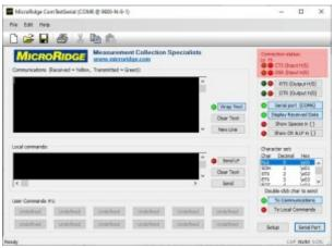
5. For the MY KEY SERIAL 2 you should be able to toggle the transmitter keying output with the RTS or DTR buttons below the status indicators.
