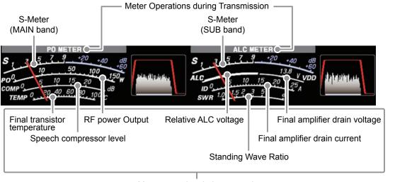
Meter operation during transmit
