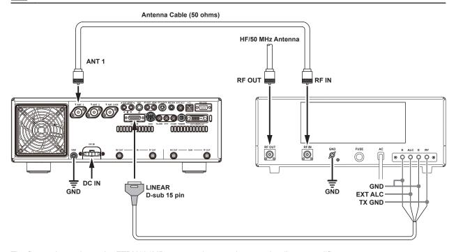
The figure above shows the FTDX101MP rear panel connections to other linear amplifiers.
