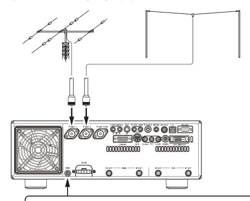
To prevent damage from lightning, atmospheric electrical discharges, electric shock etc., provide a good earth ground. Use a short, thick, braided cable to connect the station equipment to the buried ground rod (or alternative earth ground system).
