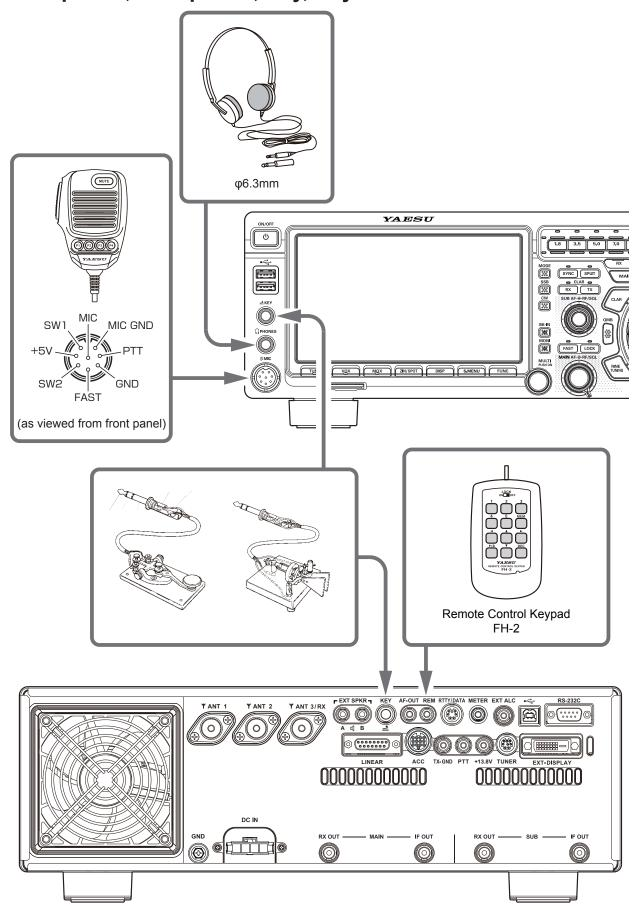
Key-up voltage on the front key jack is approximately +3.3 V DC, and key-down current is approximately 1 mA. Key-up voltage on the rear key jack is approximately +5.0 V DC, and key-down current is approximately 3 mA.
