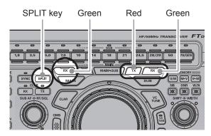
During Split operation, the MAIN band register will be used for reception, while the SUB band register will be used for transmission. If you press the [SPLIT] key once more, Split operation will be cancelled.
