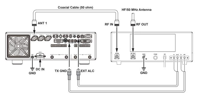
The figure above shows the FTDX101MP rear panel connections to other linear amplifiers.
