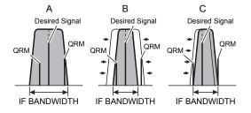
For best interference reduction, the WIDTH and SHIFT features are the primary tools you should use, after narrowing the bandwidth (WIDTH) and/or adjusting the center of the passband (SHIFT). The Contour control may then yield additional signal-enhancement benefits on the net residual bandwidth. Even more, the IF NOTCH Filter (described later) may also be used, in conjunction with these filter systems, to significant advantage.
