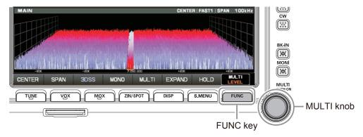
Press the [FUNC] key to call up the function screen for setting various functions. The setting menu (page 88) is also called from the function screen. Press again to return to the normal operation screen. Touch a MENU item, or rotate the [MULTI] control knob to make a selection.
