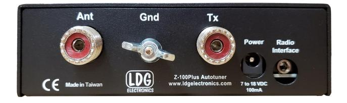
Ant: Connect the 50 ohm coax antenna feedline to this standard SO-239 connector.
